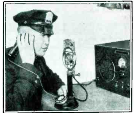
Dispatching over W2XAT, a spectacular experimental police radio station operating on "UHF" (60 MHz) in 1934.
